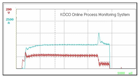
Graphics of a stud welding process with 16 mm shear connectors. Current, time and voltage are instantaneous values at the position of the cursor; welding time and energy are valid for the whole cycle.
