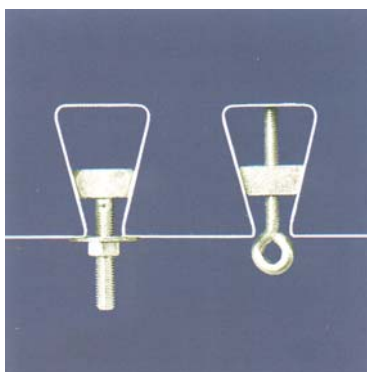
Figure 7: Attachments to the grooves of trapezoid sheets
